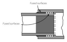
Fused and bonded surfaces of joined pipe and fitting
