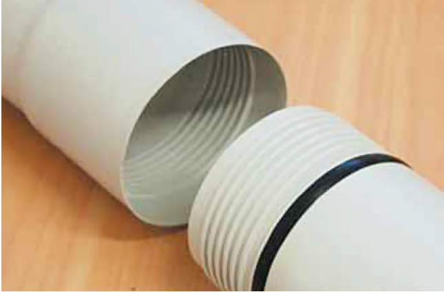
Figure 1 Typical joint arrangement showing the rubber sealing ring, threaded spigot and “low profile” threaded socket.
