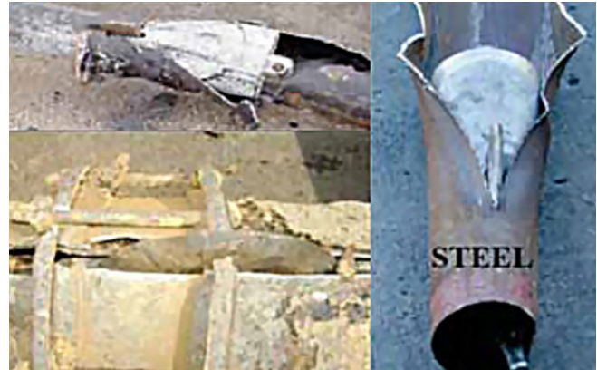
Figure 8.9 Typical "steel wheel" or "blade" type bursting heads.
