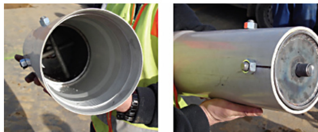
Figure 7.2 Typical DN150 Internal Pull Head.
