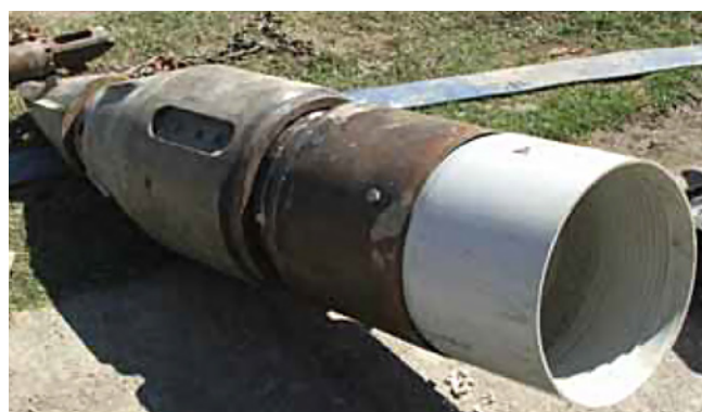
Figure 8.11 Typical External Bursting Head. DN300 Restrain™ Sewer Pipe.
