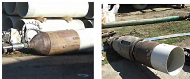
Figure 7.3 Typical DN300 External “Cone Style” Pull Head.
