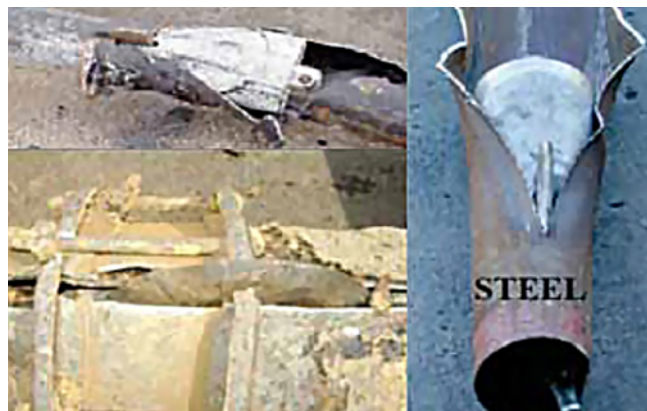
Figure 8.9 Typical "steel wheel" or "blade" type bursting heads.
