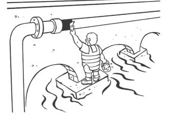
Hey, black pipes are the best to use outdoors cos black reflects the ultra violet rays better. U.V. attacks coloured PE pipe real quick! If you need to use striped or colour skin pipe for some reason, paint 'em with a light coloured acrylic paint... The light colour paint will reflect the heat in those hot summer months.
