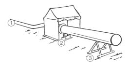
Clamp up and align your pipe ends to ensure the two pipe spigots are evenly aligned around the entire circumference of the pipe. Most machines have adjustable jaws to correct out of round pipe.
