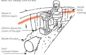
Compacted granular bedding/aggregate surrounds the pipe and up to a minimum 100mm above the pipe. Then I use selected ordinary backfill. I compact with my machine below, beside and above the pipe in layers of 300mm until I get to the top surface.
