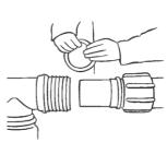
3. Insert the pipe into the body of the fitting until it meets the interior step of the fitting body. Then draw the seal ring and the bushing close to the body of the fitting.
