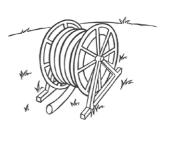
Here's another way to do it... 125mm PE pipe made into coils then placed onto a pipe dispensing trailer.
