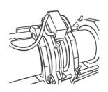
Wait for the cooling time to pass. Then inspect the joint for consistency. The fusion bead should look like the McDonalds M. Check your data logger recordings, then make a **go or no**
