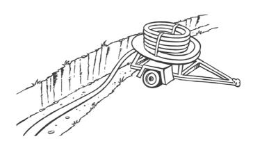
I've done a bit of pipe bursting in my time too, that's one of those in-line replacement trenchless technology methods where you have an ol' water main that you want to rehabilitate without using 'dig n lay' methods. I get Iplex to make coils of 125mm PE pipe and get it made straight onto carousels like this......
