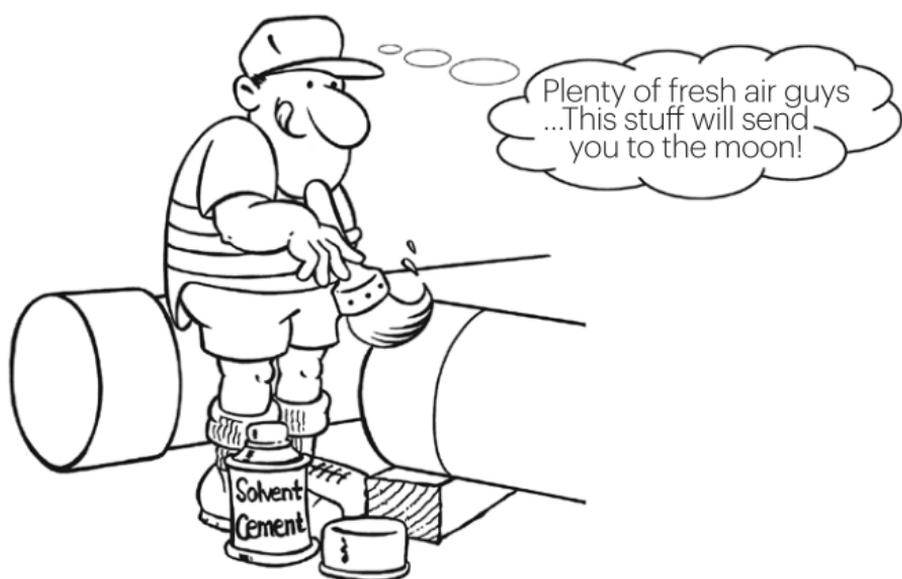
I put one even thick coat inside the socket then a thicker coat on the spigot. I use the large brush I bought; my mate Willy helps me as well. Don't hang around – **move quickly...** If the cement looks dry before jointing – **give the dry parts another coat!** It must not dry before I get it together.
