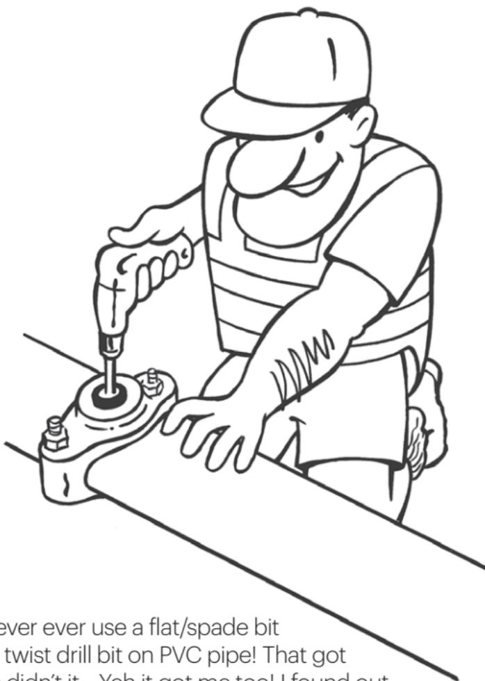
Never ever use a flat/spade bit or twist drill bit on PVC pipe! That got ya didn't it... Yeh it got me too! I found out the hard way. I now use a **sharp** fine tooth hole saw - it never lets me down! (Make sure it stays sharp!)
