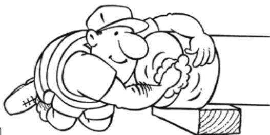
Rest the pipe socket on a piece of timber; get all the dirt and grime out of the socket.
