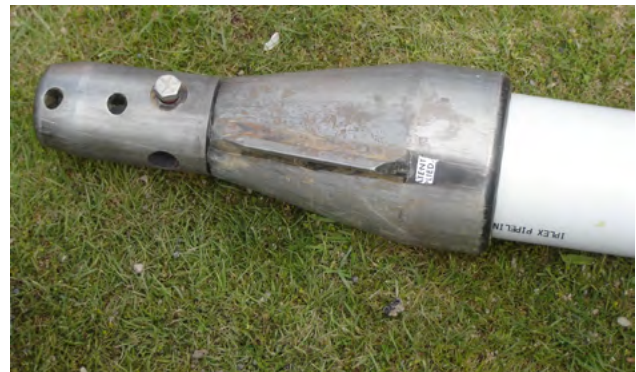
Figure 7.9 Typical External "Cone Style" Bursting Head. Upsize of existing 100mm CI pipe with new PVC pipe.
