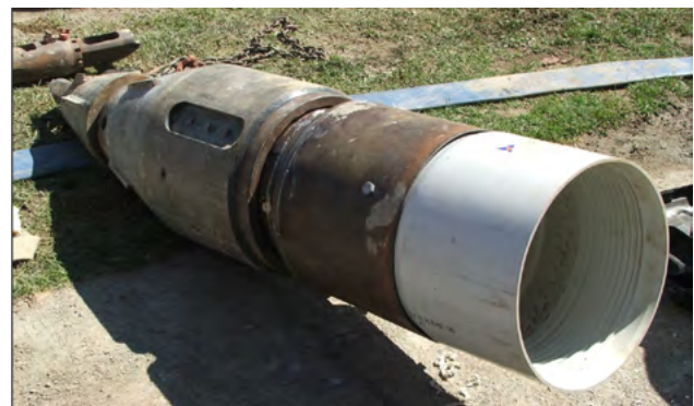
Figure 7.10 Typical External Bursting Head with DN300 Restrain® Starter Pipe.
