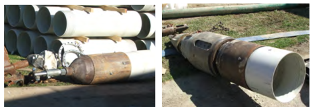
Figure 6.4 Typical DN300 External 'Cone Style' Pull Head
