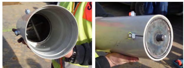
Figure 6.3 Typical DN150 Internal Pull Head
