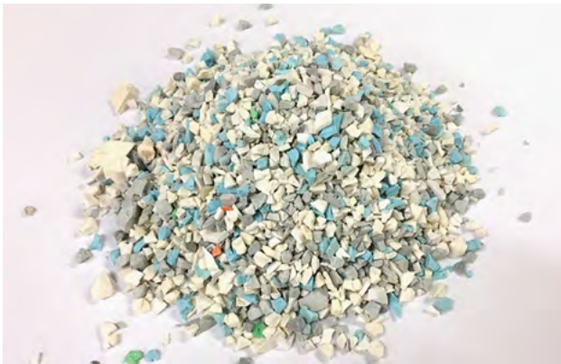
Figure 6.6 - Mixed PVC pipe recyclate material in chipped form ready for reprocessing
