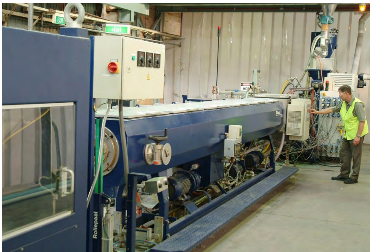
Extrusion Equipment used for the manufacture of Iplex Apollo® PVC-O Pressure Pipe
