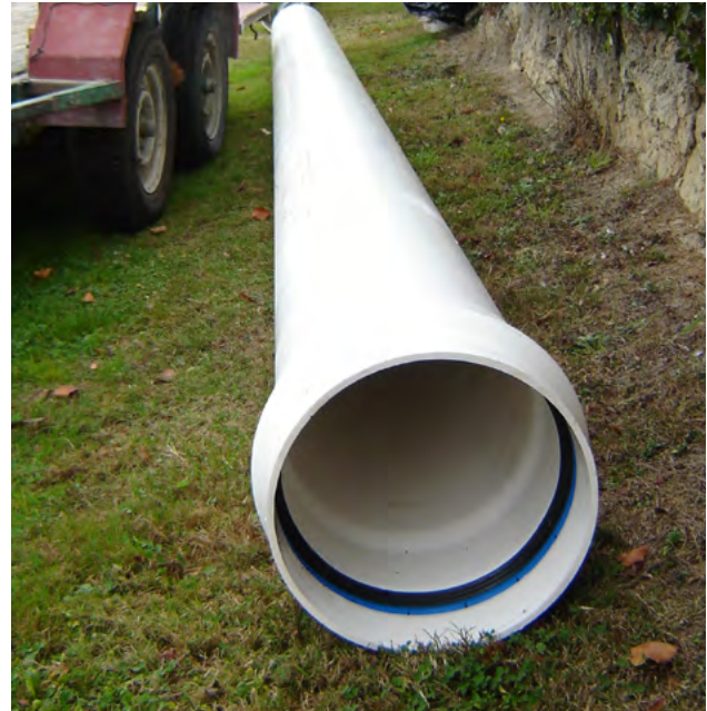
Figure 4.3 - Joint socket on white DN 300 Series 1 PN 12.5 Iplex Apollo® PVC-O pipe, with factory fitted, retained Anger-lock™ seal ring
