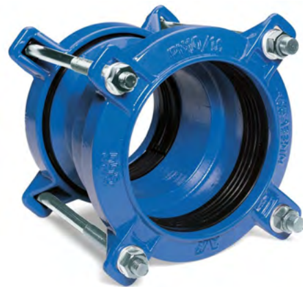
Figure 9.10 - "AVK" brand Series 601 PN 16 Universal Couplings for DN 100 PVC-O, pressure pipe. The range of allowed compatible pipe OD sizes is moulded on the end cap
