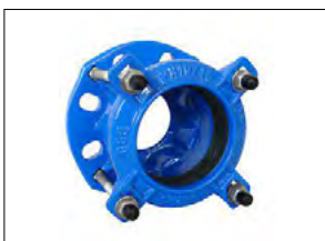
Figure 9.9 - "AVK" brand Series 603 PN 16 Universal Flange adapters suitable for Appollo PVC-O, pressure pipe. The pressure rating (PN 10 /16) and range of allowed compatible pipe OD sizes is moulded on the end cap
