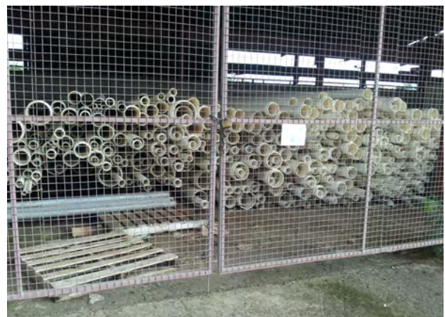
Figure 11.4 - Long term storage, under secure cover for PVC pressure pipe, - Apia, Western Samoa
