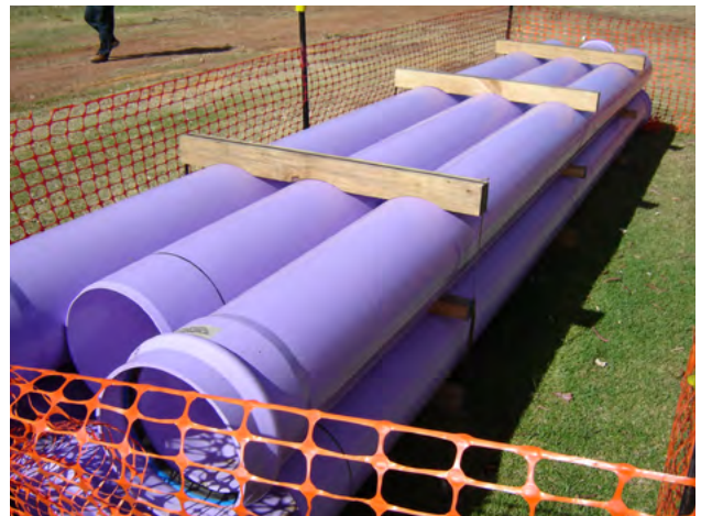
Figure 2.3 - Iplex Apollo® PVC-O DN 300 Series 2 PN 16 PVC-O pipe, coloured lilac for non potable recycled water application, Adelaide, South Australia
