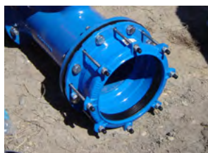
Figure 9.9 - "AVK" brand Series 603 PN 16 Universal Flange adapters suitable for Appollo PVC-O, pressure pipe. The pressure rating (PN 10 /16) and range of allowed compatible pipe OD sizes is moulded on the end cap
