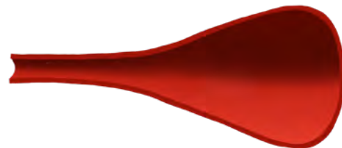
Figure 3.4 - Wall cross-section of "pre-form" pipe with a small diameter and a large wall thickness being stretched circumferentially and axially into a pipe with larger diameter and a thinner wall
