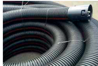
Iplex NEXUS HI-WAY pipe coil showing the pull-out resistant coupling and red stripe for visual identification
