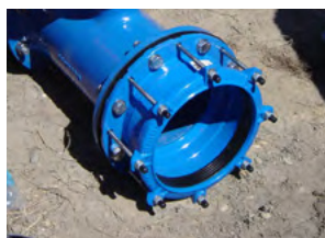
Figure 3.8 - "AVK" brand Series 603 PN16 Universal Flange adapters suitable for Iplex® PVC, pressure pipe. The pressure rating (PN10/16) and range of allowed compatible pipe OD sizes is moulded on the end cap
