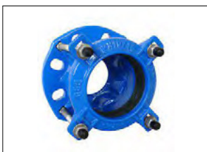
Figure 3.8 - "AVK" brand Series 603 PN16 Universal Flange adapters suitable for Iplex® PVC, pressure pipe. The pressure rating (PN10/16) and range of allowed compatible pipe OD sizes is moulded on the end cap
