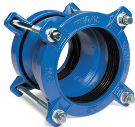
Figure 3.9 - "AVK" brand Series 601 PN16 Universal Couplings for DN100 PVC pressure pipe. The range of allowed compatible pipe OD sizes is moulded on the end cap
