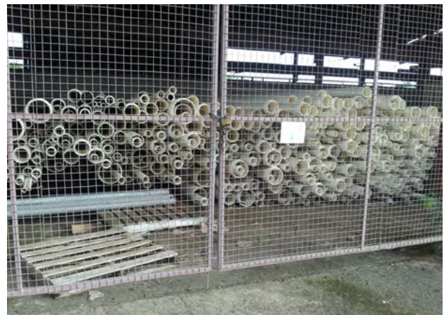
Figure 6.4 - Long term storage, under secure cover for PVC pressure pipe, - Apia, Western Samoa
