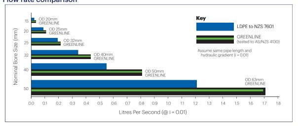
Note: The information contained in this flow comparison is intended to be of a general nature. It should be used as a guide only, and not for Design. Before relying on any of the information in this brochure, you should first consult Iplex Pipelines NZ.
