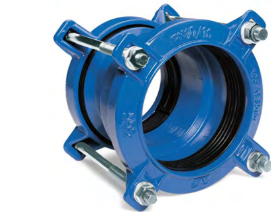
Figure 4.9 - "AVK" brand Series 601 PN16 Universal Couplings for DN100 PVC-O, pressure pipe. The range of allowed compatible pipe OD sizes is moulded on the end cap
