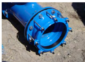
Figure 4.8 - "AVK" brand Series 603 PN16 Universal Flange adapters suitable for Appollo PVC-O, pressure pipe. The pressure rating (PN10/16) and range of allowed compatible pipe OD sizes is moulded on the end cap
