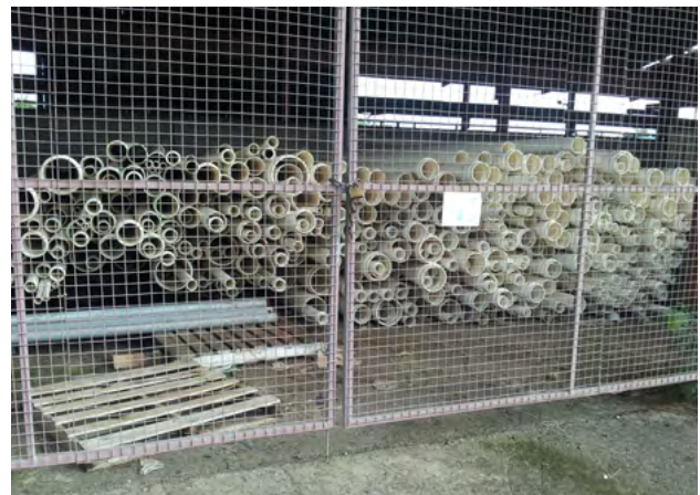
Figure 7.4 - Long term storage, under secure cover for PVC pressure pipe, - Apia, Western Samoa
