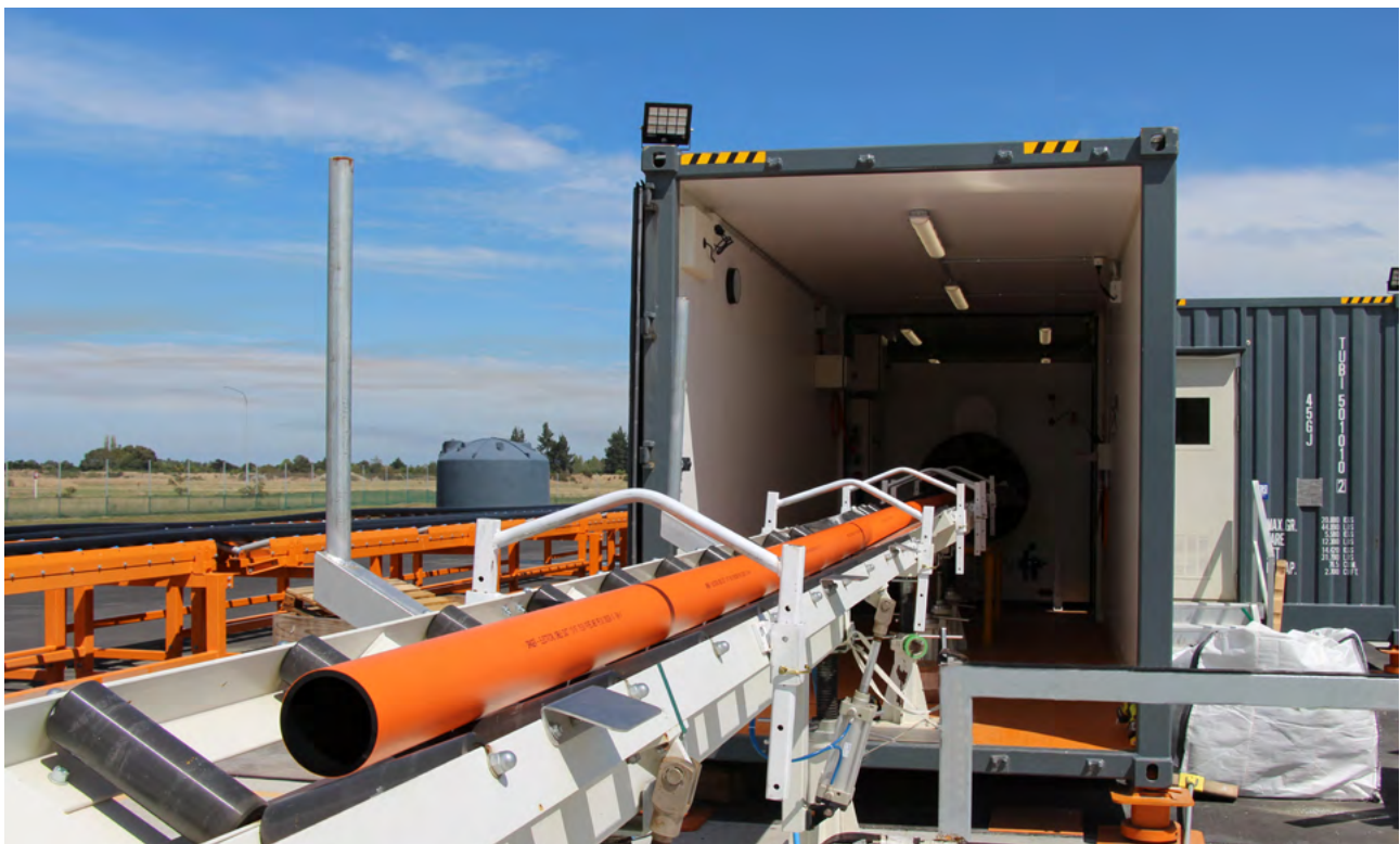
Iplex® PE Duct being extruded at the Iplex® Ashburton plant.
