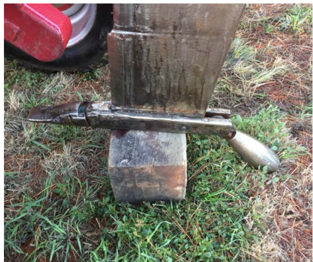
Mole plough, blade, torpedo and plug
