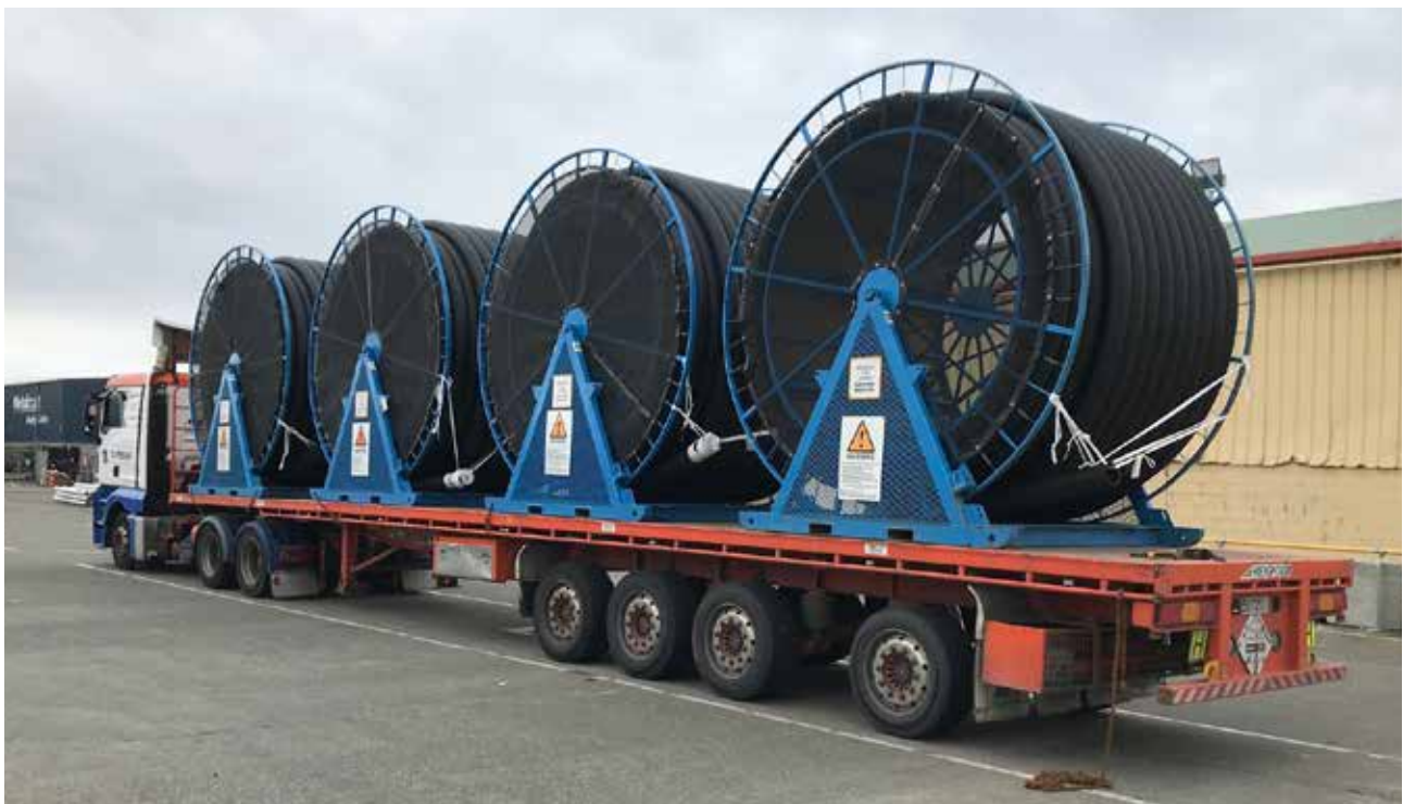
Image 12. Drum Coils on truck showing strapping – DO NOT remove strapping until ready to be dispensed.
