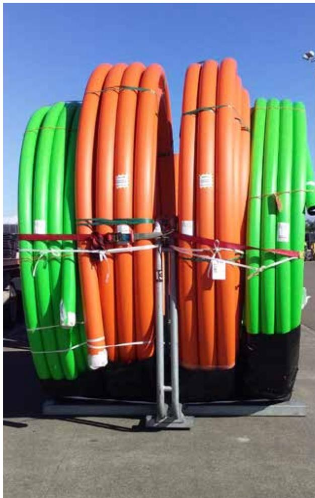
Image 7. Large free standing coils attached to the transport stand.
