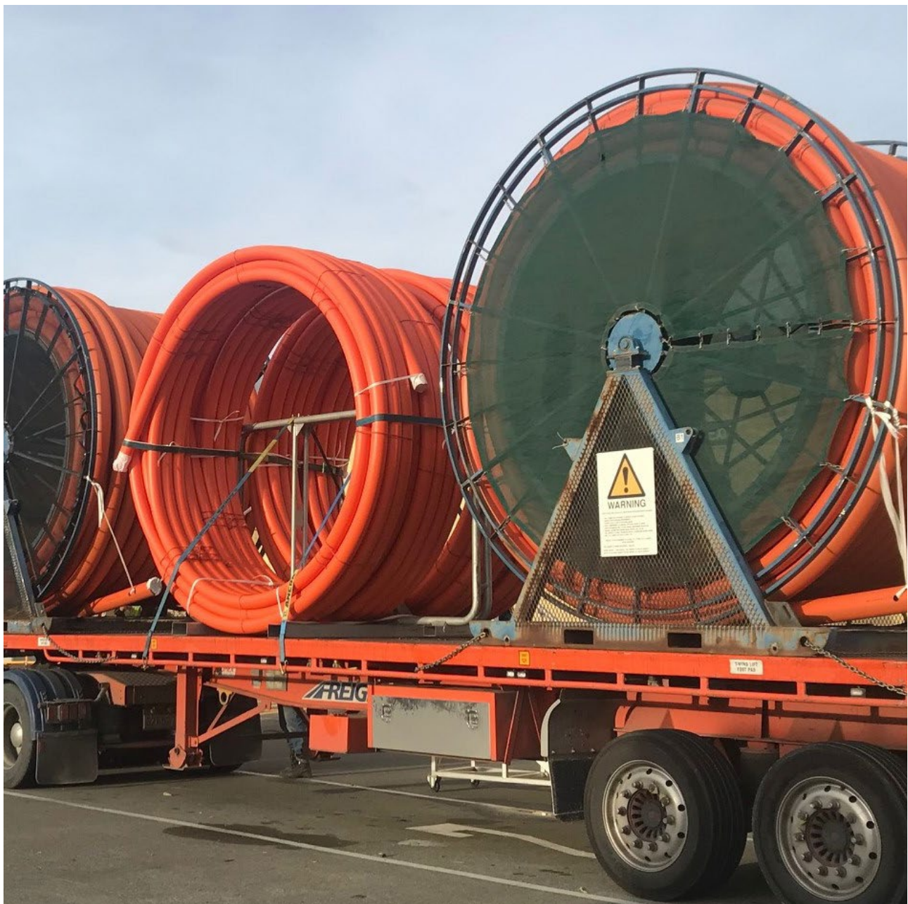
Iplex DN 110 SDR 17 PE Flexible Electrical duct in Free Standing coils and Drum Coils
