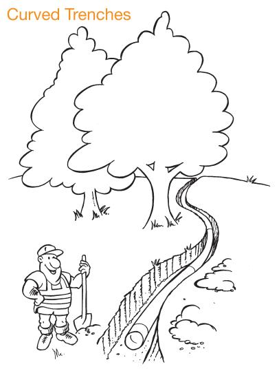
PVC pipe becomes more flexible once joined into a pipe-string. For curved trenches, join the pipe above ground in a straight line then lower it in - 'snaking' it in carefully as you go. The larger the pipe diameter the larger the curve, the rule of thumb for a radius of curvature is 300 times the outside diameter of the pipe!
