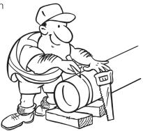
I measure the pipe socket inside and subtract 5mm to make it shorter. This is the witness mark measurement. The witness mark should be just visible
