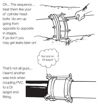
The nut end of the bolt must always be on the DI casting cos the nut end takes up the load first. If you don't you may damage the pipe.
