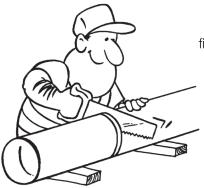
I always cut pipe using a fine-tooth hand saw, it's much easier with blocks of wood under each pipe. Y 'can use a petrol power saw with an abrasive disk too. A witness mark is needed on the spigot (plain) end of the pipe to:
