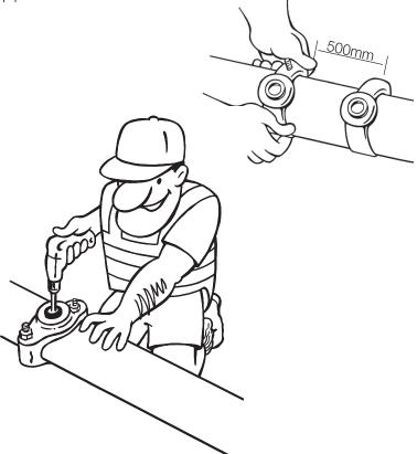
Never ever use a flat/spade bit or twist drill bit on PVC pipe! That got ya didn't it... Yeah it got me too! I found out the hard way. I always use a fine tooth hole saw or shellcutter - they never let me down! (Make sure the hole saw or shellcutter stays sharp!)
