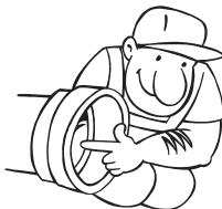
All PVC pipe needs a full circle pipe-stop to rest the pipe up against when installing to prevent over-insertion.
