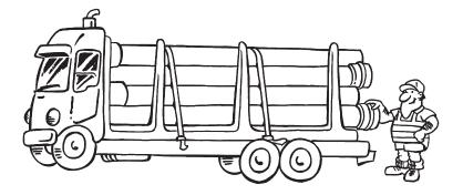
Y'know – you've got to look after these PVC pipes. They **must NOT** roll around the truck deck and the socket ends must stick out and be protected to avoid damage.
