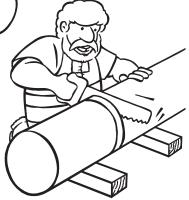
An electric chainsaw is OK too but if you plan on any **HOT** fusion jointing then you should never use a chainsaw with the chain oil function operating cos the oil stuffs up ya' fusion (welded) joint. You are better off replacing the saw's blade and chain more often than have a whole heap of failed fusion joints on a job somewhere!
