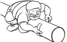
strapping to wrap around the pipe then mark off using a piece of Kiwi ingenuity...a piece of number 8 fencing wire! A white crayon will work fine too.
