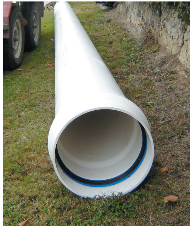
Joint sockets on white DN 300 Series 1 PN 12.5 Apollo pipe, with factory fitted, locked in place blue seal rings.
