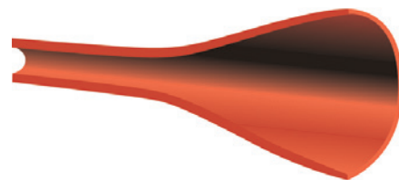
Figure 4: Wall cross-section of “pre-form” pipe with a small diameter and a large wall thickness being stretched circumferentially and axially into a pipe with larger diameter and a thinner wall.
