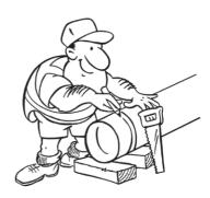
I measure the pipe socket inside and subtract 5mm to make it shorter. This is the **witness mark** measurement. The witness mark should be **just visible** once installed.
