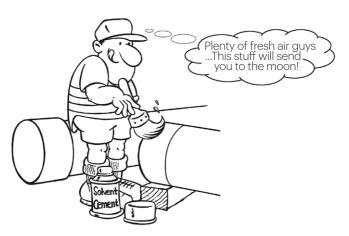
I put one even thick coat inside the socket then a thicker coat on the spigot. I use the large brush I bought; my mate Willy helps me as well. Don't hang around – **move quickly...** If the cement looks dry before jointing – **give the dry parts another coat!** It must not dry before I get it together.
